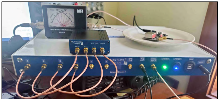
Figure 2. The 'Beacon-Blaster-6' prototype #2 from Turn Island Systems, capable of simultaneous FSK transmissions on six bands from 1.8 MHz to 50 MHz. Image from https://turnislandsystems.com/beaconblaster-progress/
