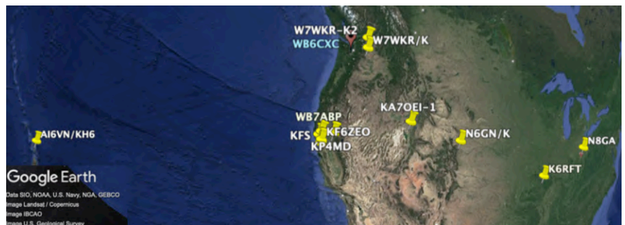
Figure 3. Map showing the transmitter site at WB6CXC, Friday Harbour, WA, and the KiwiSDR receiver sites with useful data on one or more bands. The marker for KPH in the San Francisco Bay area is hidden.
