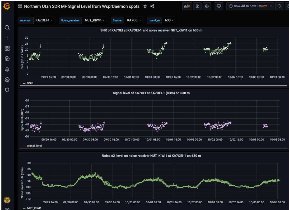
In this example, on 630 m, the receiver is the Northern Utah SDR site as KA7OEI-1 and the Sender is KA7OEI at a distance of 115 km. It is reasonable to assume that propagation is via ground (surface) wave, and that, as a consequence, the signal level should be essentially constant with time.
