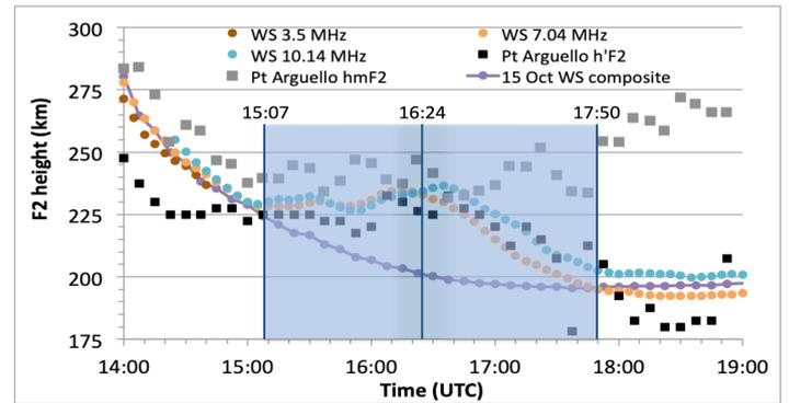
Figure 3. An expanded view of F2 heights time series with the composite tri-frequency WSPRSONDE trace for 15 October. The shaded area shows start, mid and end times of the eclipse at the earth's surface.
