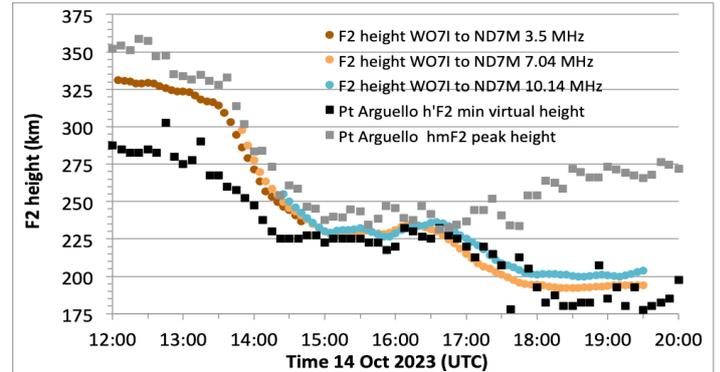
Figure 2. Time series of ionosphere F2 heights from Pt Arguello ionosonde and from WSPRSONDE at 3.5, 7 and 10 MHz on a 545 km path 87-89% obscured by the eclipse. The average of h'F2 and hmF2 at 15:00 was the seed for forward and backward integration of path velocity from the WSPRSONDE.
