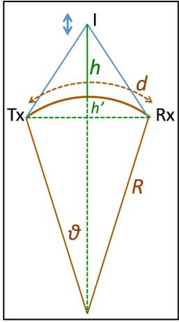
Figure 1. Diagram to show path length and hmF2 height calculations. Not to scale.
