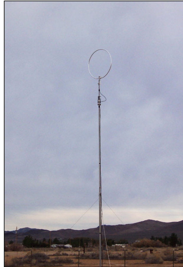
ND7M, S. Nevada: Wellbrook ALA1530LN Magnetic Loop via 250' Heliax -> BCB -> LNA (20dB) -> splitter->HPF & T1-1-X65X 40-10m KiwiSDR ->LPF & T1-1-X65X 2200-60m KiwiSDR
