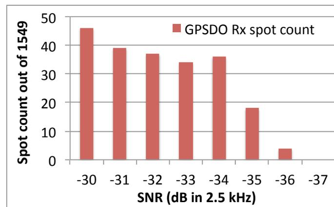
Test null hypothesis of no difference in count of SNR  $\leq$  -30 dB FST4W-300 spots decoded by receivers with phase-lock GPSDOs and standard KiwiSDR GPS aiding. Phase-lock GPSDO Tx at 7 MHz at N6GN.
