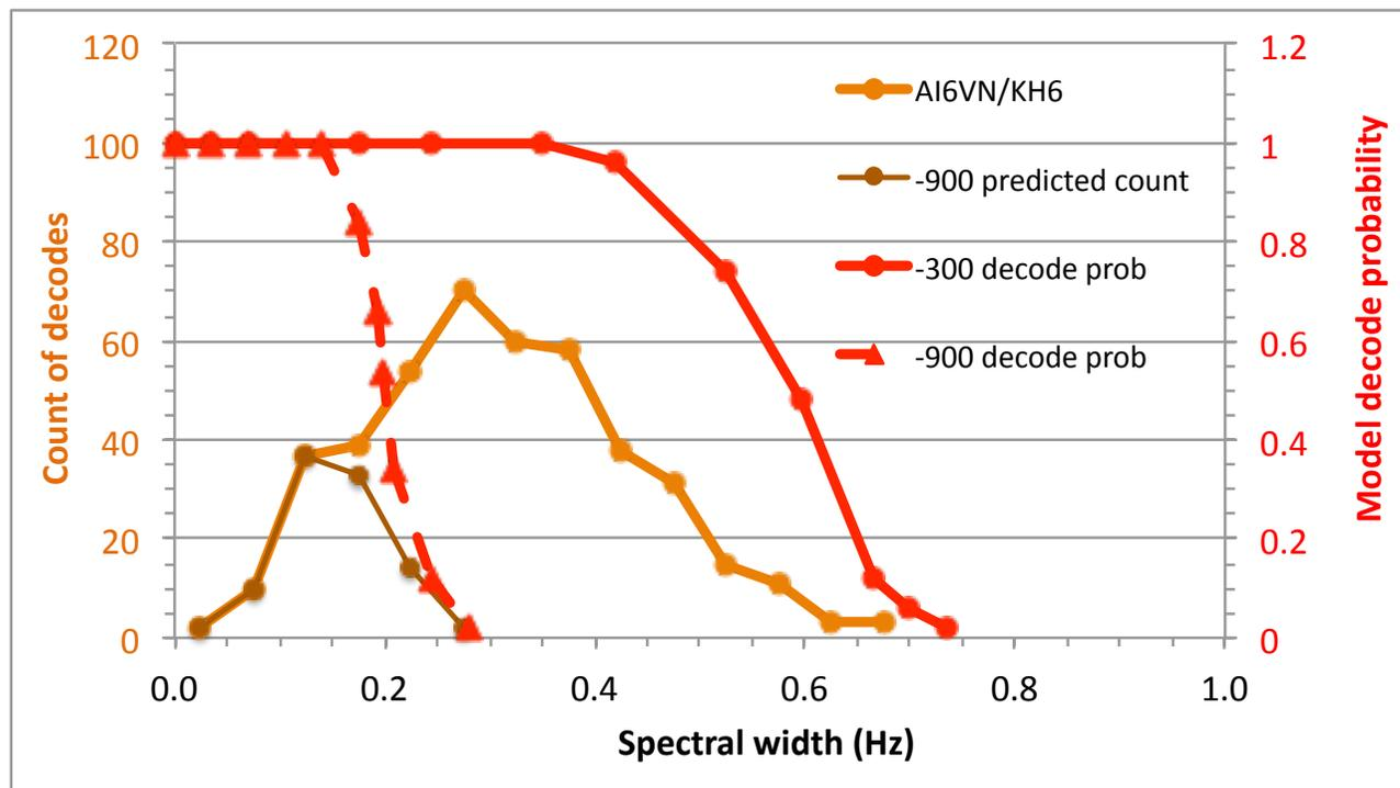
From FST4W-900 *fst4sim* decode probability (dashed red) and measured spectral width (orange) we'd expect few spots (brown) to be decoded over this path. In fact we received very few.
