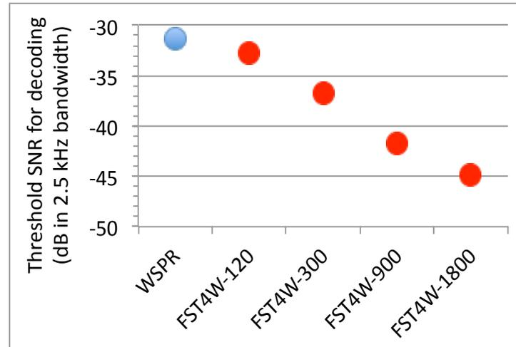
Defined at 50% probability of decode with Doppler spread of no more than 0.01 Hz
