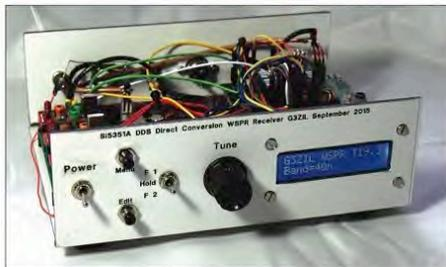
The author's latest version, in development. This uses the main board as described in the article plus an Arduino clone with a QRP Labs Arduino shield and a QRP Labs S15351A synth for the local oscillator. It covers up to five bands with a QRP Labs relay switched board with the author's own size-compatible plug-in single-crystal filters.
